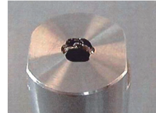
Orifice worn out by slurry
