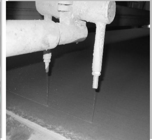
Cleaning effect, minimal maintenance, quality improvement, reduce wasted water, energy savings, and more... IKEUCHI's CERJET® spray nozzles help solve various problems in paper & pulp making process as indispensable tools.
