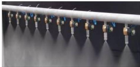
Spray header with KB nozzles assembled
